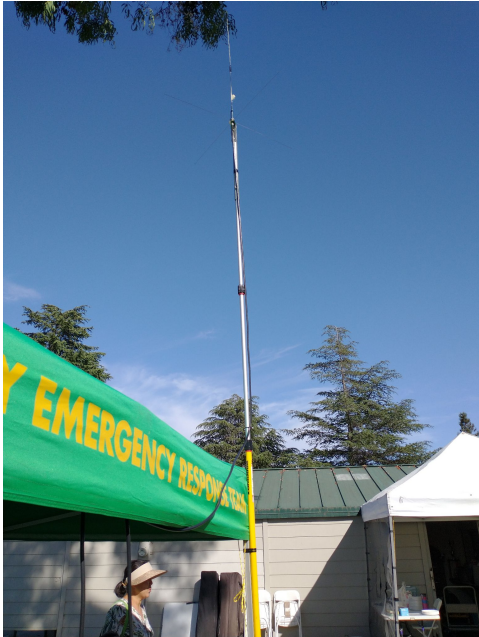
Base antenna on extendable painter's pole
