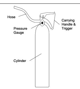
Components of a portable fire extinguisher: Hose, carrying handle and trigger, pressure gauge, cylinder
