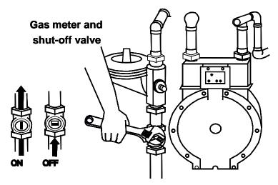
The gas meter shutoff diagram indicates the shutoff valve location on the pipe that comes out of the ground. To turn off the valve, use a non-sparking wrench to turn the valve clockwise one-quarter turn. Remember that, in all cases, natural gas flow should only be turned on by a licensed technician.
