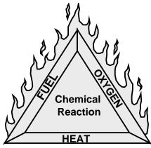
Fire Triangle: Fuel, oxygen, and heat create a chemical reaction, which causes fire.
