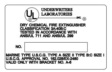
Sample manufacturer's label for a fire extinguisher, showing the Underwriters Laboratories symbol at the top, the type and classification of fire extinguisher, testing procedures used, and serial number. At the bottom of the label is marine information, including the U.S. Coast Guard approval number.
